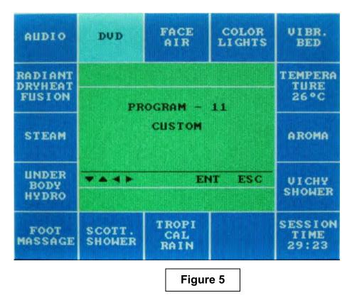
You can change and adjust all available (visible) functions with the touch of a finger on the control panel. Programs 1 - 10 are preset programs and have selected default
