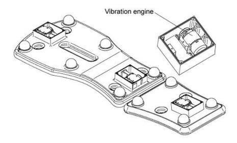
The vibration system has three (3) electrical motors. The motors are connected to special nests on the back of the beds. Two (2) motors are located on the upper bed, and one (1) motor is located on the lower bed.
