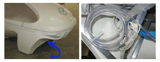
4. Release the tube from the frame by removing the plastic strip. Locate the end of the 02-IN tube and connect it with the Oxygen System.
