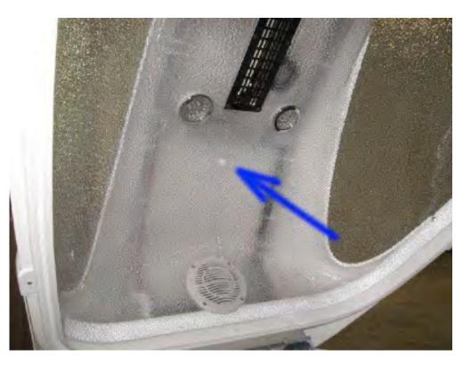
6. 02 will flow into the capsule through the 02 nozzle on the hood in the foot area as shown in the picture below.
